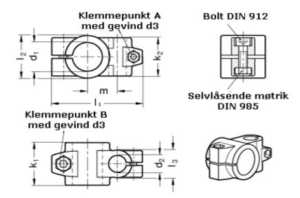
Adjustable clamp lever for d3 = GN 911-M10-55 have to be ordred separately 11 = 122.0Adjustable clamp lever for d4 = GN 911-M 8-32 have to be ordred separately 12 = 65d1 13 = 40= 48= 25 m = 45d2 = M10d3 = M 8d4 = 65 k1
